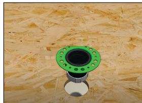
Step 1: Install Deck Flange
