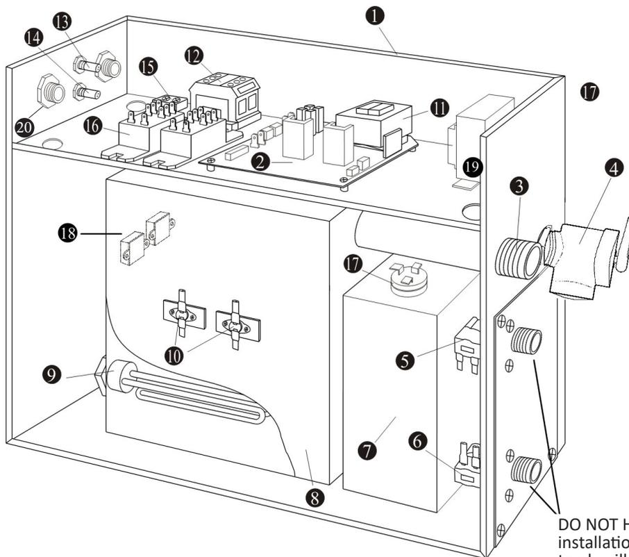
DO NOT HEAT during installation. Using a torch will cause damage to plastic solenoid valve
